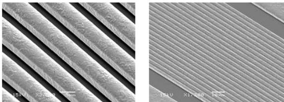
Figure 11. SEM Image of 5/5um and 2/2um LW/LS RDL
