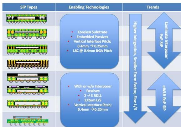
**Figure 4.** SiP Vertical Integration Technologies
