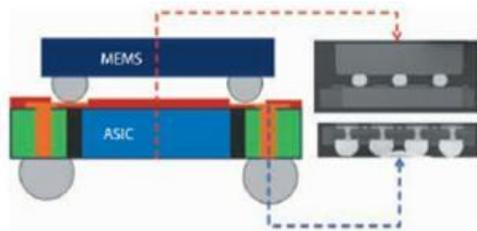
**Figure 7.** 3D eWLB for MEMS/Sensor Devices [2]
