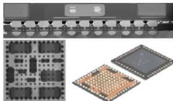
**Figure 5.** 3D SiP eWLB-PoP with Discrettes in Interposer on Top Package
