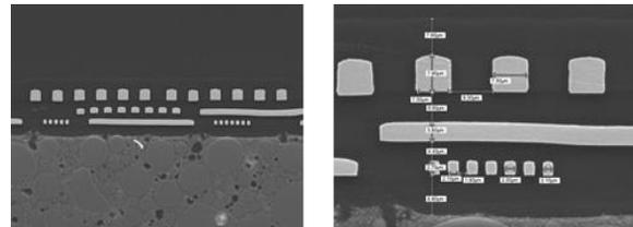
Figure 12c. SEM image of 3-Layer RDL eWLB Test Vehicle
