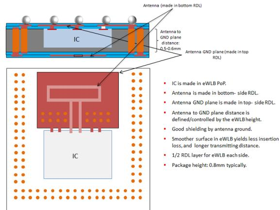
**Figure 8.** Double Sided RDL eWLB AiP Module
